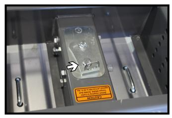
7. Torque the top bolt to 60 ft/lbs and install the locking bracket over the top bolt and secure in place.
