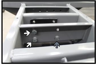
3. Install the four (4) 1/2"-13 x 1-1/2" bolts with lock washers thru the hitch into the plates (white). Install the two (2) 1/2"-13 x 3/4" bolts with lock washers thru the hitch into the plates (gray). Torque the six (6) bolts to 78 ft/lbs, then remove the 1/2"-13 x 4-1/2" bolt installed previously.
