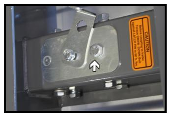
6. Install the 1/2"-13 x 1-1/2" top bolt thru the hitch into the shank. Align the plastic pads per manufacturer's instructions.
