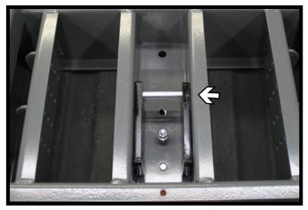
Install the adapter plates into hitch channel. Loosely install the 1/2"-13 x 4-1/2" bolt towards the rear of the hitch to hold the plates in position.
