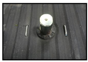
Install the hitch shank into the gooseneck hitch. Insure the flats of the shank are parallel to the bed ribs.
