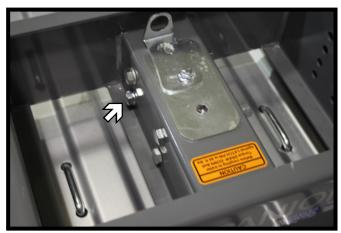
5. Install the hitch onto the shank. Install the 1/2"-13 x 4-1/2" bolt thru the hitch and shank with a lock washer and nut on the opposite side. Torque the bolts to 78 ft/lbs.
